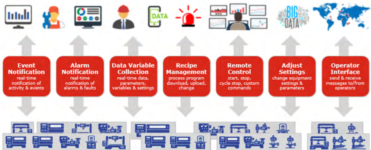
Figure 1: Connectivity architecture providing smart manufacturing functionality.
