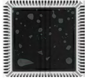
Figure 20: Typical QFN voiding for Paste D.
