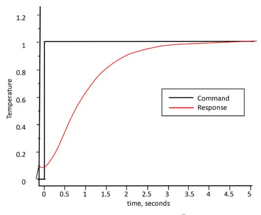
Figure 4: On-off control response [1].
