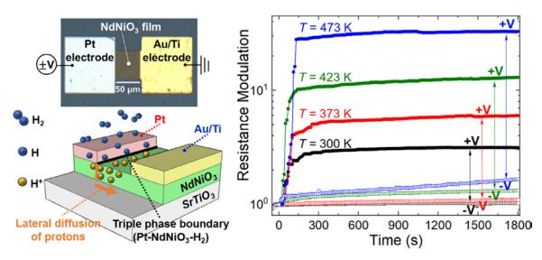
Strongly correlated oxide proton resistor devices.
