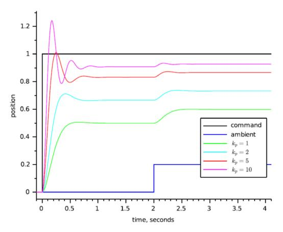
Figure 5: Temperature controller with proportional feedback. The kink at time = 2 is from the external disturbance [1].
