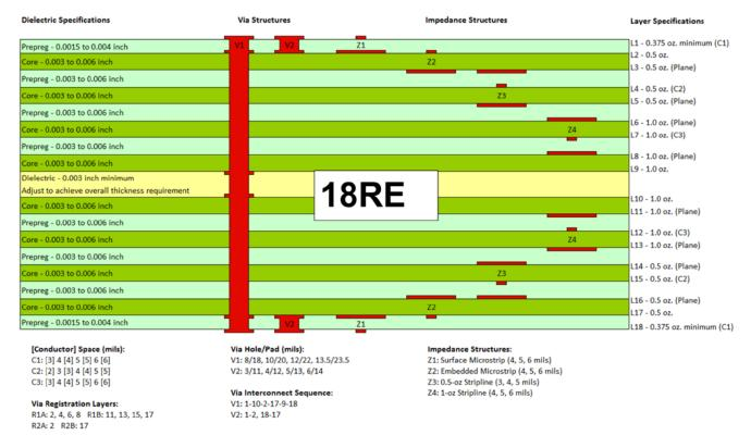
Figure 2: 18R-E panel stackup and via/trace structures.
