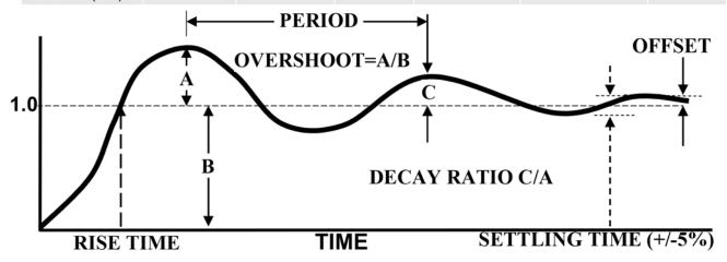
Figure 3: Characteristics of common controller responses.
