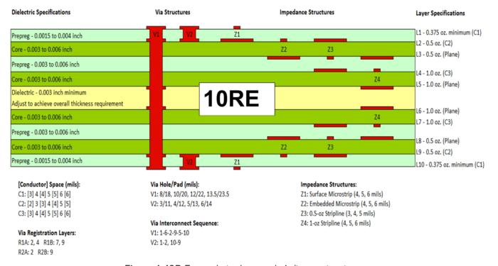
Figure 1: 10R-E panel stackup and via/trace structures.
