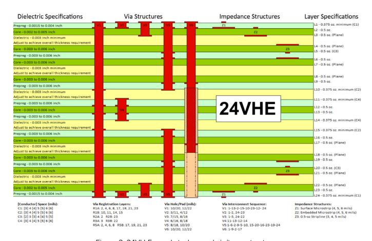
Figure 3: 24VH-E panel stackup and via/trace structures.
