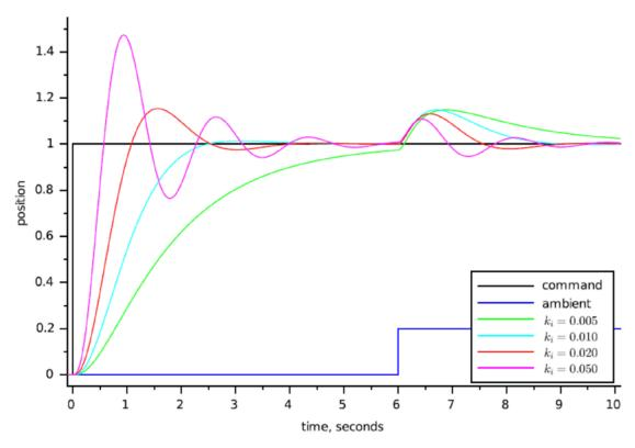
Figure 6: Integral control response. Motor and gear with proportional feedback position vs. time [1].
