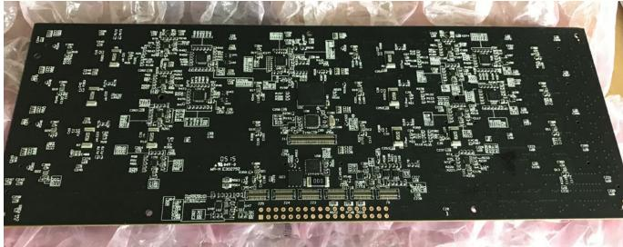
Figure 1: Photos showing the top and bottom of the CCAs that overheated due to a simple footprint error. Note the backplane controller BGA in the center of the bottom side of the board; this one CCA represents \$5,000 out the window.
