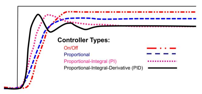
Figure 2: Control response dynamics to a change in setpoint.
