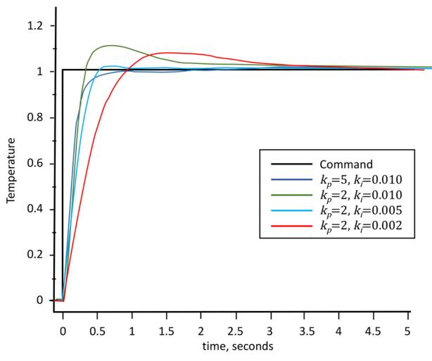
Figure 8: Response of the precision actuator system with PID control. This system settles in less than half a second compared to multiple seconds for other systems [1].
