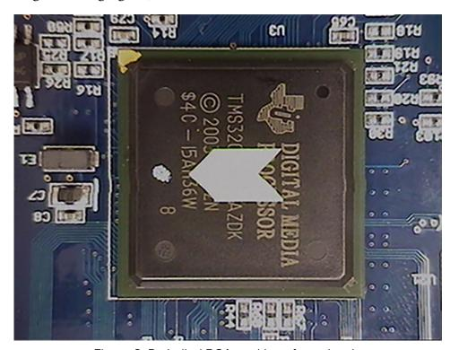
Figure 2: Re-balled BGA marking after salvaging.
