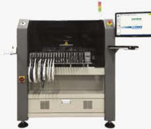
Pick & place with 160 feeder ports and 6,400 CPH placement
