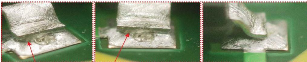
Figure 16: FOD observed between SOT lead and solder fillet in red highlighted area from Figure 15.
