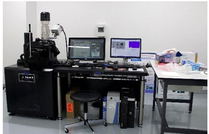
Figure 2: Scanning electron microscope.
