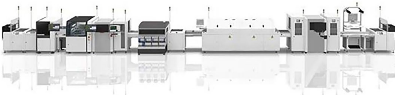
Figure 1: Two key inspection processes monitor SMT lines: SPI and AOI.
