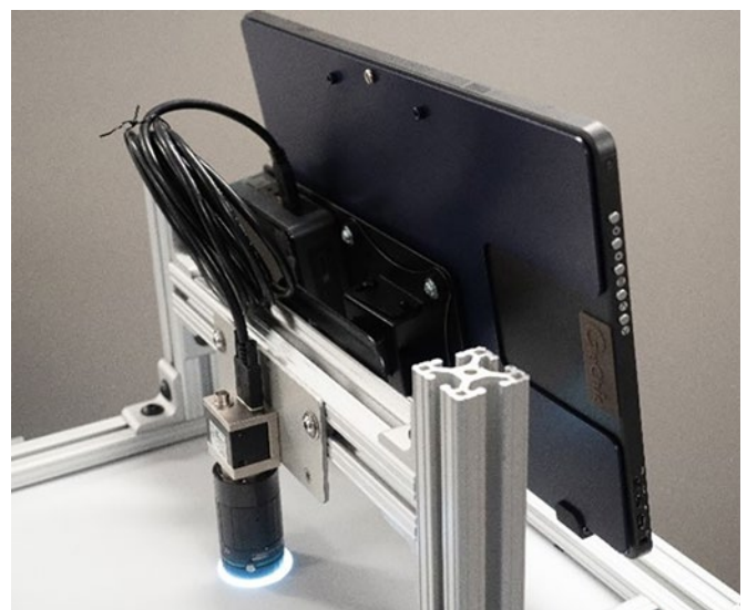
Figure 2: Standard industrial cameras, lenses, and lighting are used to capture images while standard PCs, monitor, and keyboard can be used to run the camera service.
