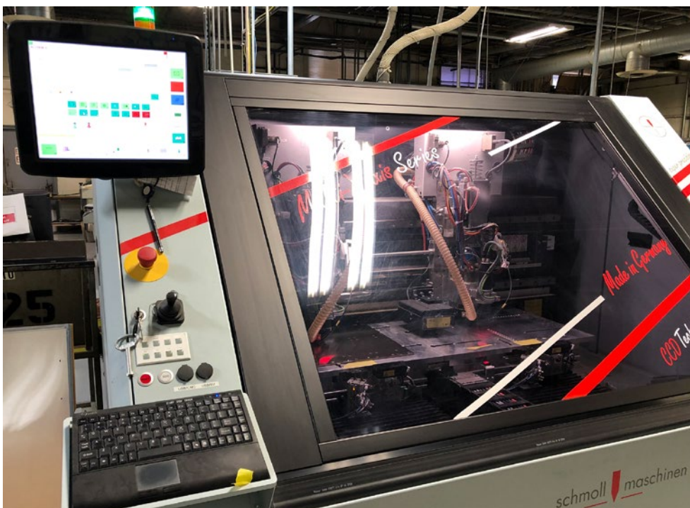
Schmoll MXY drilling machine with CCD camera for highest precision.
