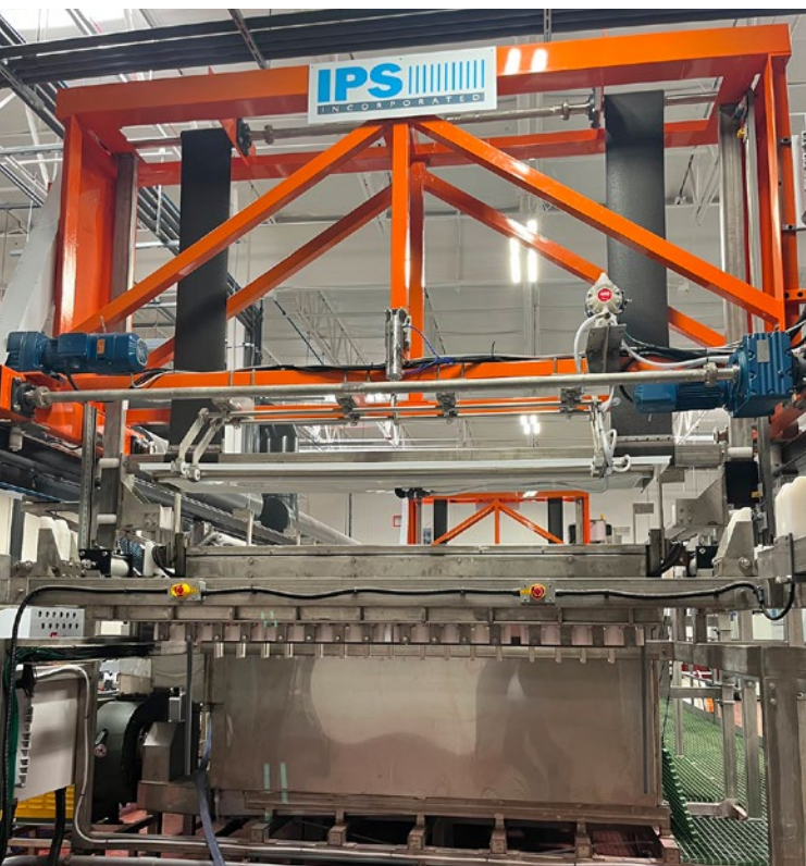
Custom Integrated Process Systems plating line with insoluble anodes for copper via fill technology.
