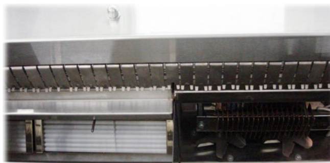
Figure 5: Example of preheaters in a wave solder system.
