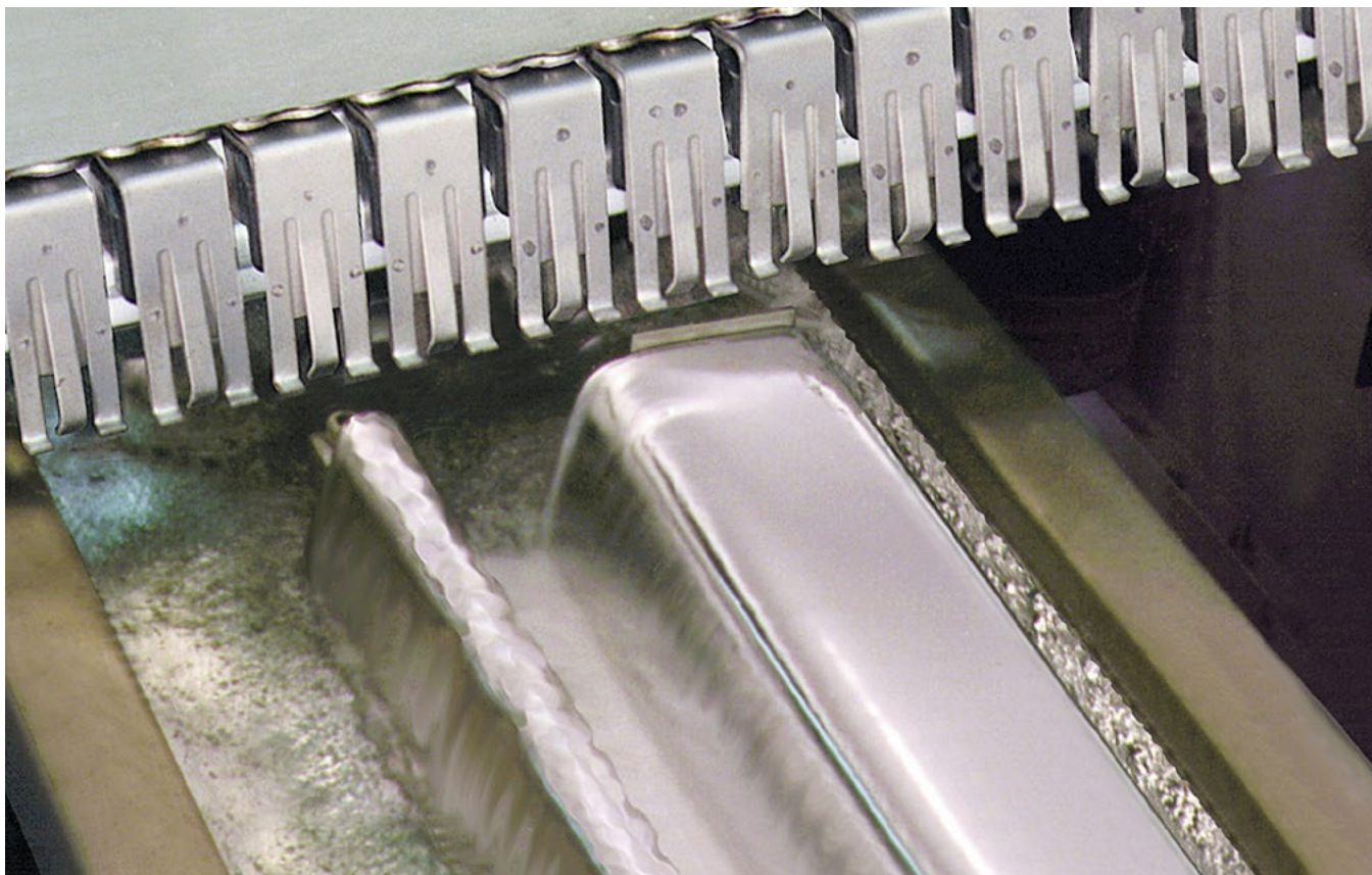
Figure 1: Turbulent wave (left) and laminar wave (right) in same system.
