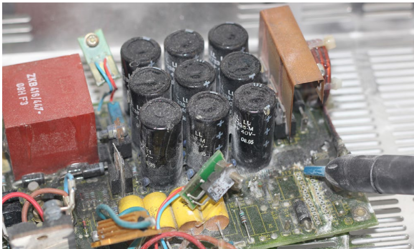
Figure 2: Microabrasion on a PCB.
